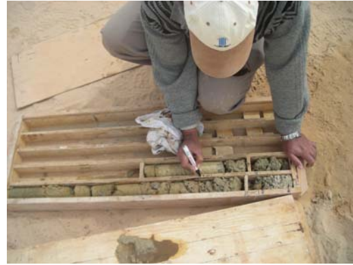
Both rigs at work, Borehole #1 in background, and Borehole #2 in foreground (left). Recording the levels of the recovered core from Sahabi Borehole #1 (right)
