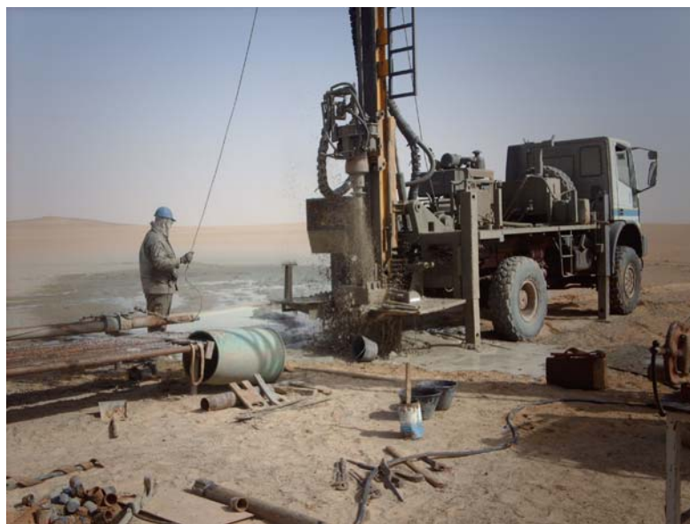
The R50 Rotamec hammer drilling rig at Sahabi Borehole #2.
