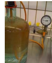
Infusion pressure is 0.2- 0.4 bar
